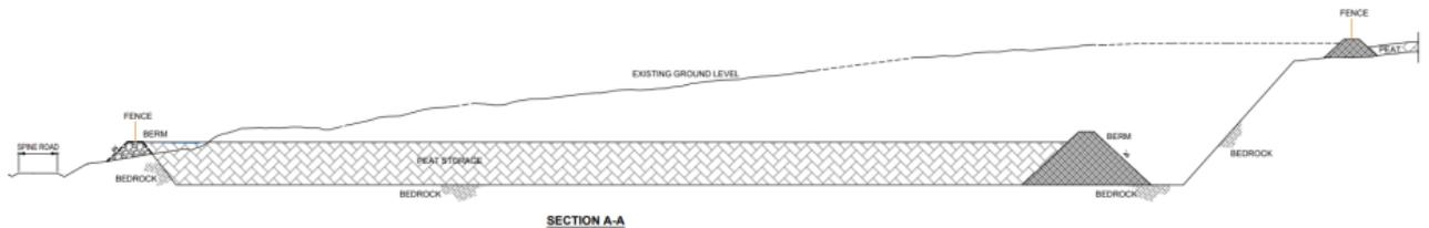
Figure 3-2 Cross Section of Borrow Pit South of Turbine 12
