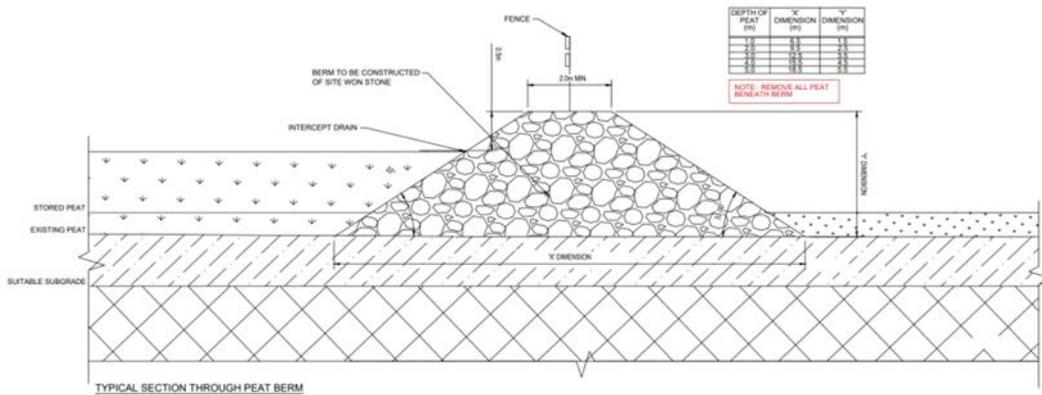
Figure 3-5 Cross-Section of a Peat Cell retaining Berm
