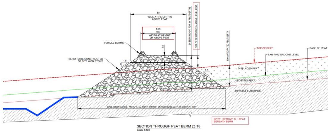
Figure 3-6 Cross Section of Peat Containment Berm
