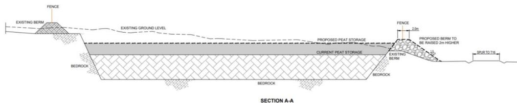
Figure 3-4 Cross Section of borrow pit between Turbine 13 and Turbine 16
